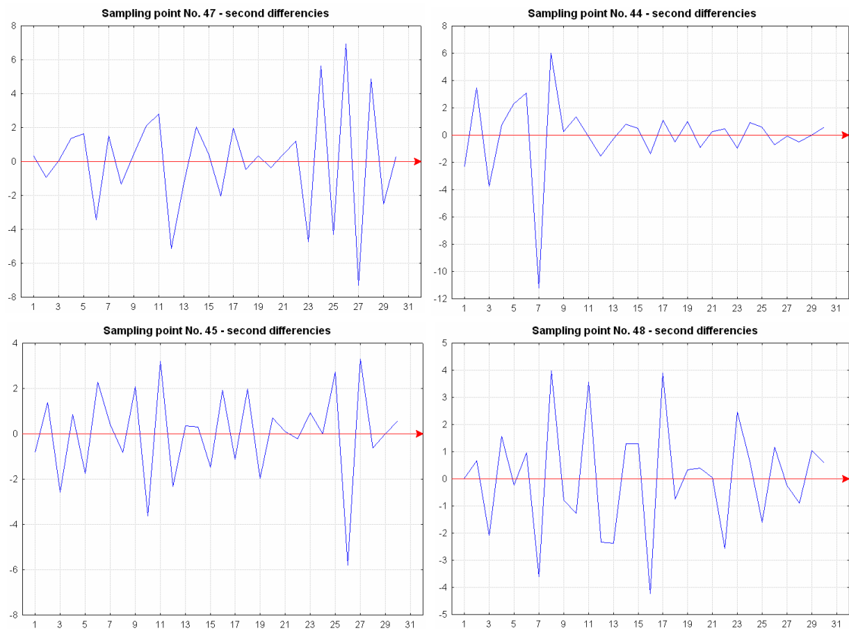
Fig. 6. A sample of second differences of ground radon volume activity. Different shapes of chart indicate various responses to weather conditions.
