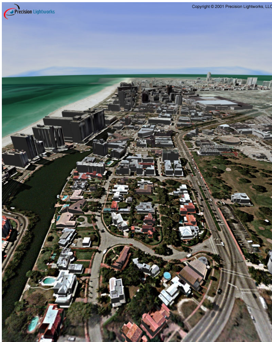
Fig. 10 Precision Lightworks Nverse Photo is a plug-in for Autodesk VIZ or Discreet 3ds max that enables users to generate 3D city scenes and data from aerial photos without the need for stereo viewing hardware.
