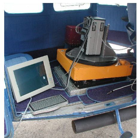
Figure 1: AISA Eagle VNIR airborne hyperspectral system mounted in the aircraft.
