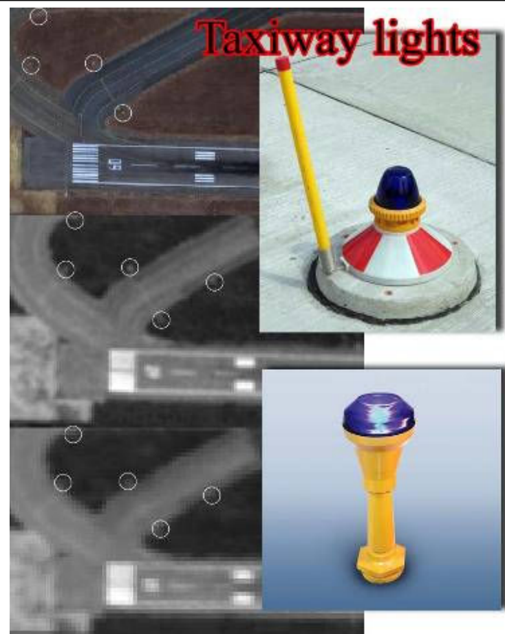
Fig.3. Taxi way lights marked with white circles on images with resolution: 1 m (on the top), 2,5 m and 5 m.
