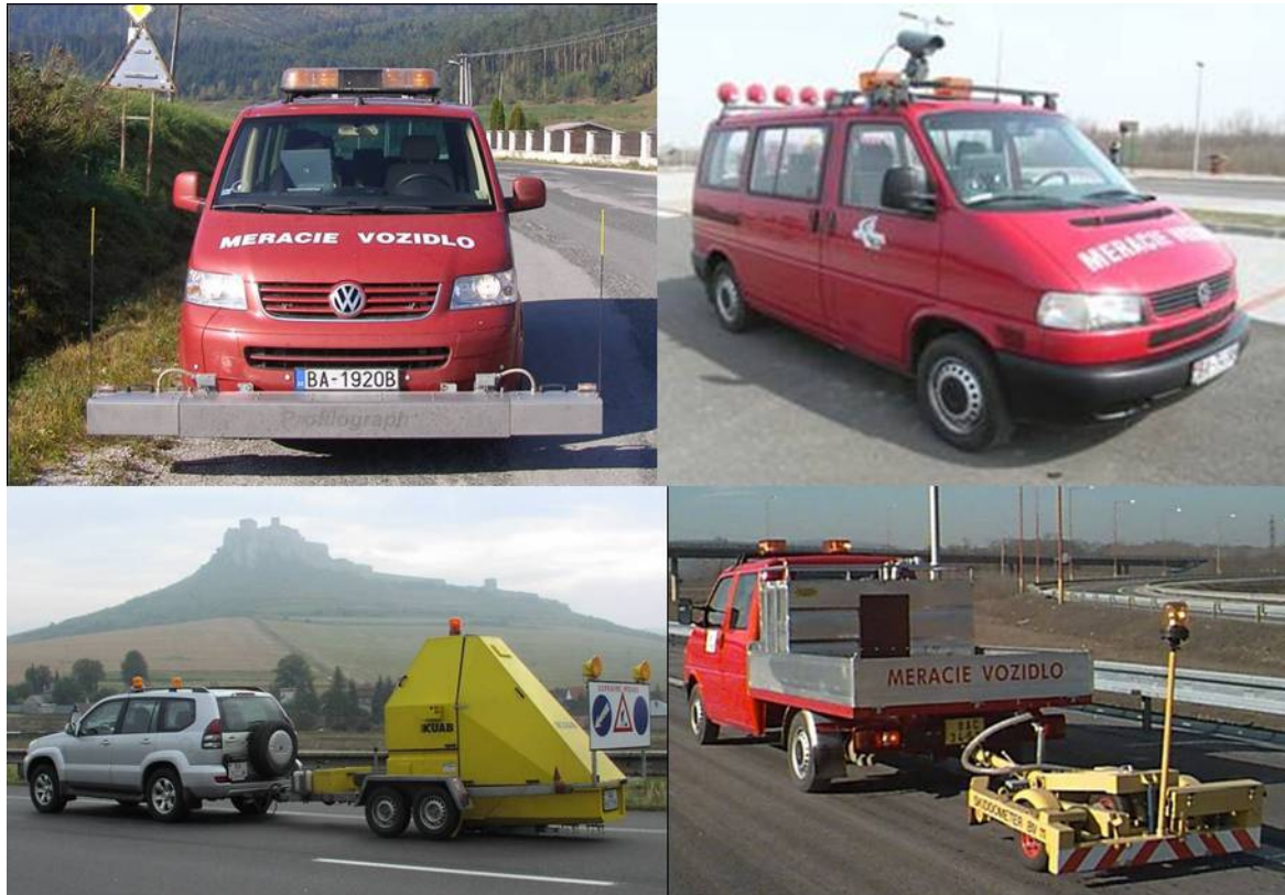
Obr. 3 Zariadenia pre diagnostiku vozoviek – Profilograph GE, Videocar, KUAB FWD50, Skidometer BV 11
