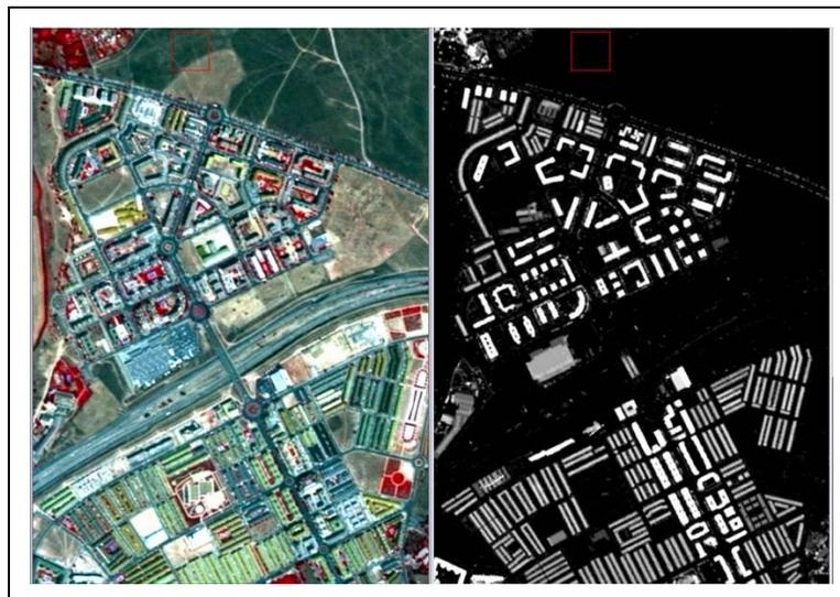
**Fig. 1** Normalized Digital Surface Model (nDSM = DSM-DTM)
