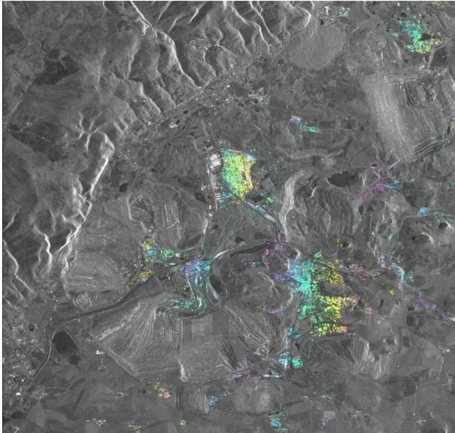
Fig. 2. Atmospheric phase (time baseline of 106 days) – value cycle of  $2\pi$
