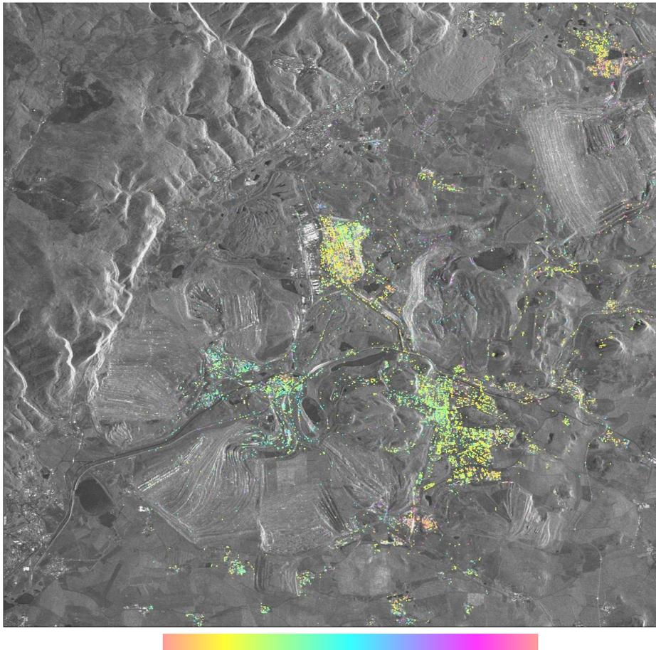
**Fig. 3.** Linear deformation (temporal baseline 106 days) – one colour cycle stands for 0,02 m (-0,01;0,01)
