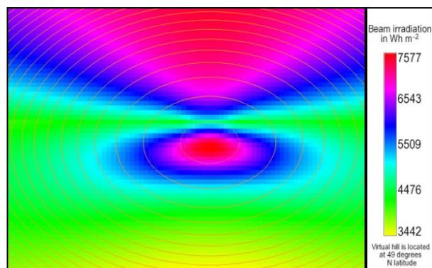
**Fig. 5** Beam irradiation (midsummer day): beam irradiation is computed by model r.sun without the shadowing effect of terrain.
