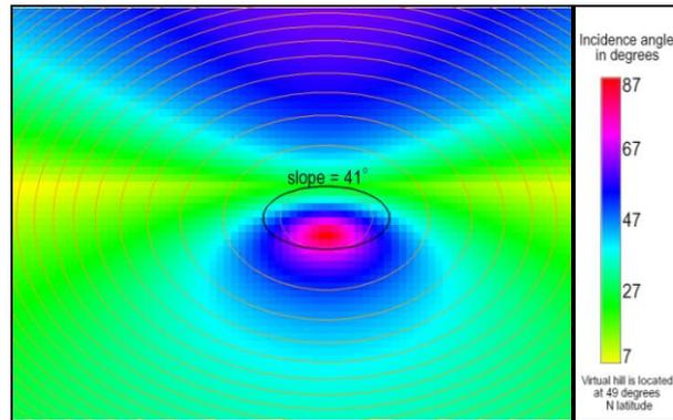
**Fig. 3** Solar incidence angle map (midsummer day at noon): incidence angle is computed by model r.sun without the shadowing effect of terrain.
