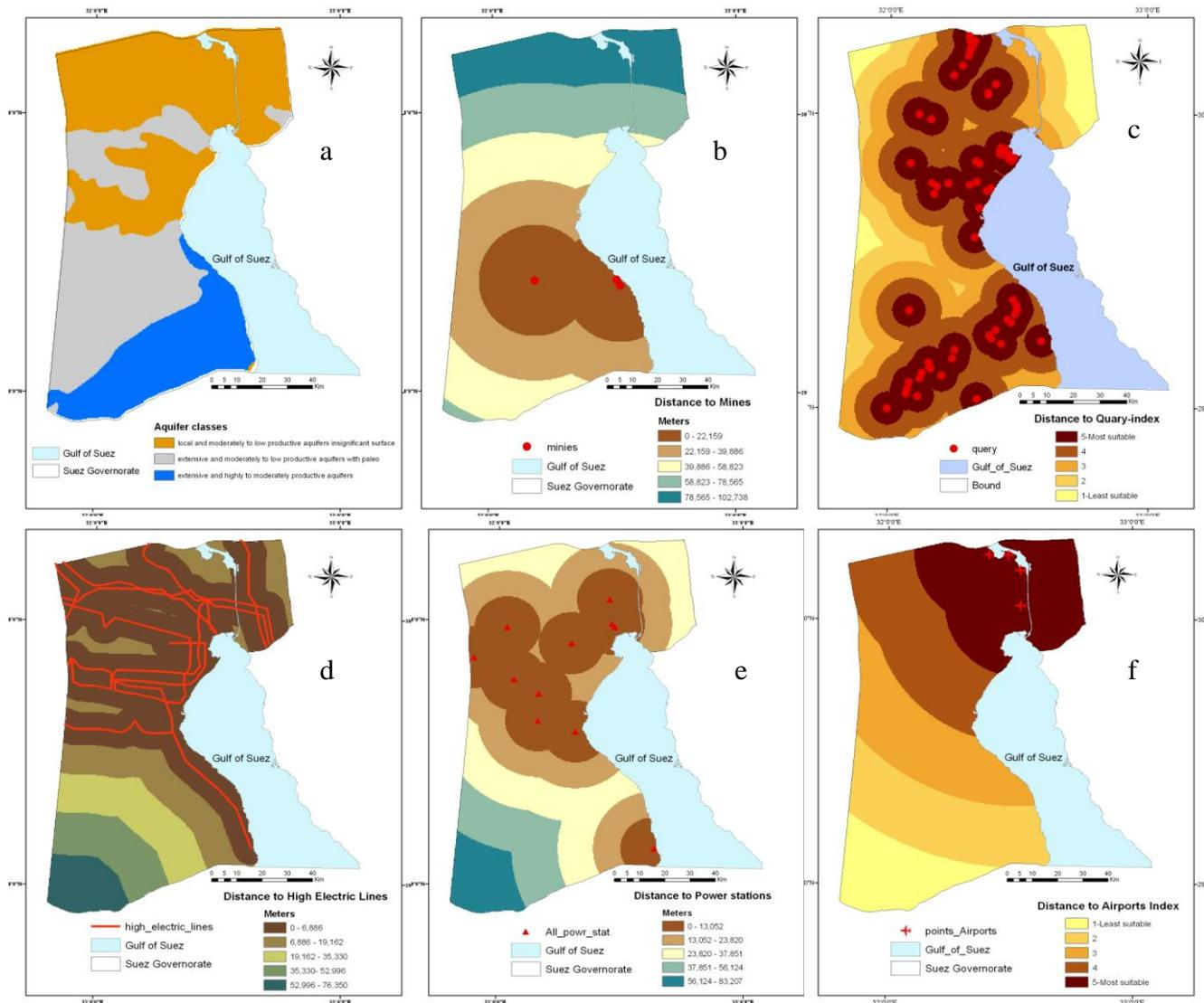
**Fig. 4.** Criteria maps for identifying zones suitable for industrial development. (a) Aquifer classes. (b) Distance to mines. (c) Distance to Quarries. (d) Distance to high electric lines. (e) Distance to power stations. (f) Distance to Airports.
