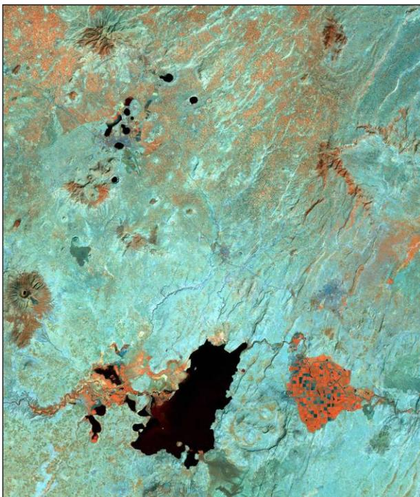
**Fig. 1.** RGB synthesis of Landsat channels 4-5-7 enhancing water bodies (dark objects), vegetation cover (red) and bare grounds (cyan)
