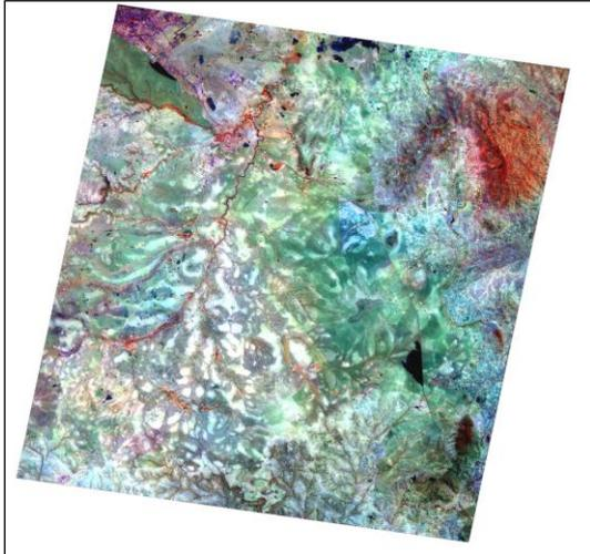
**Fig. 3.** RGB synthesis of Terra Aster channels 3-4-7 enhancing water bodies (dark objects), vegetation cover (red) and bare grounds (cyan)
