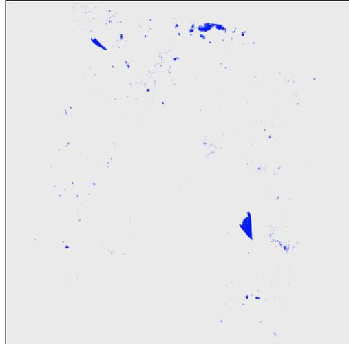
**Fig. 4.** Terra Aster scene - final mask of water bodies in Machakos region. The final mask is a combination of NDSI approach and thresholding of channel AST 3N.
