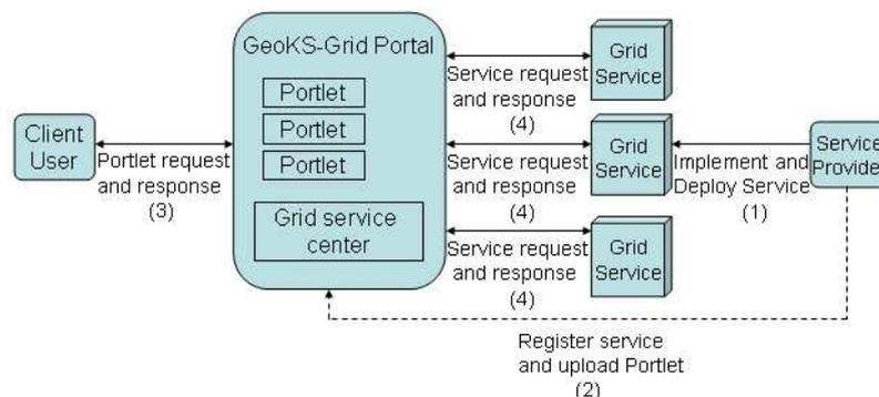
**Fig.3.** The Process of service deploy and register in GeoKSGrid
