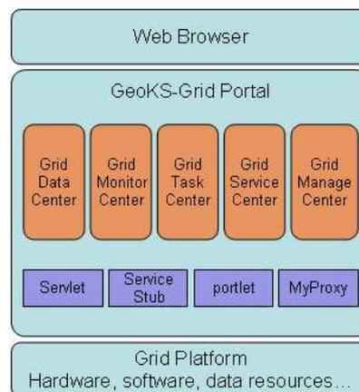
**Fig.2.** GeoKSGrid Portal Architecture
