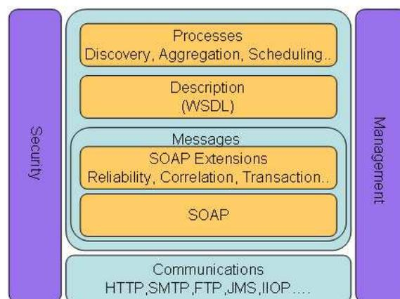
**Fig.1.** Grid Service Architecture (Source: W3C)
