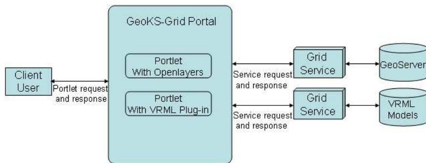
Fig.4. The services that Deployed in GeoKSGrid
