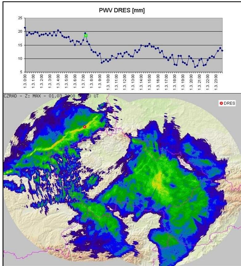
Fig. 5a: Comparison of the results got from GPS measurements at the DRES reference station with the image from meteorological radar at March 1<sup>st</sup> 2008
