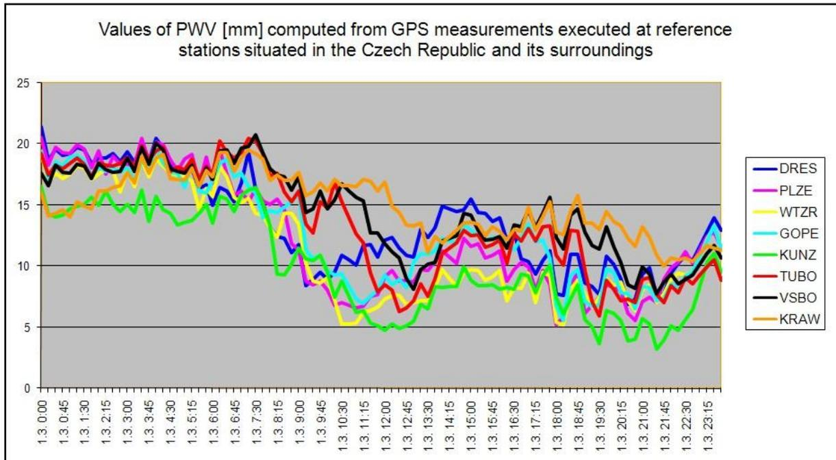
Fig. 2: PWV values [mm] for November 1<sup>st</sup> 2008 computed from data measured by GPS reference stations located in the Czech Republic and its surroundings
