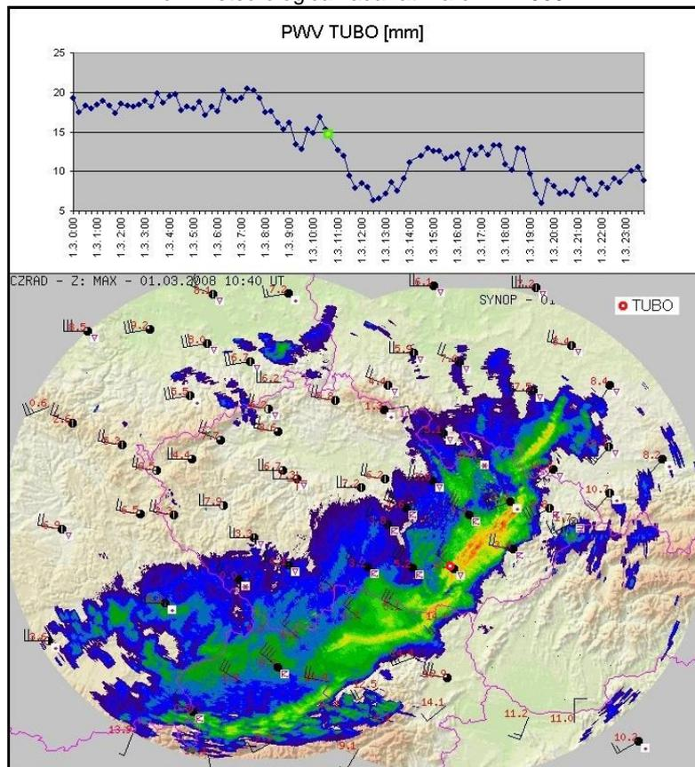
Fig. 5c: Comparison of the results got from GPS measurements at the TUBO reference station with the image from meteorological radar at March 1<sup>st</sup> 2008
