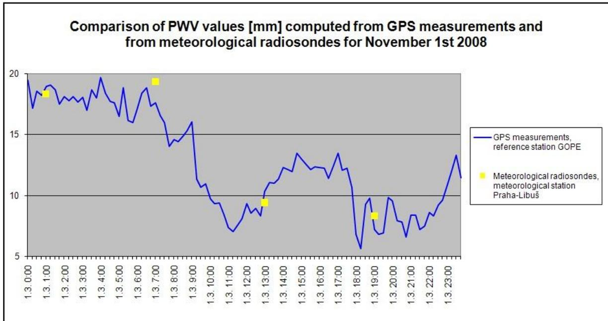
Fig. 3: PWV values [mm] for November 1st 2008 computed from data measured by GPS reference station GOPE and from meteorological radiosondes emitted from meteorological station Praha-Libuš
