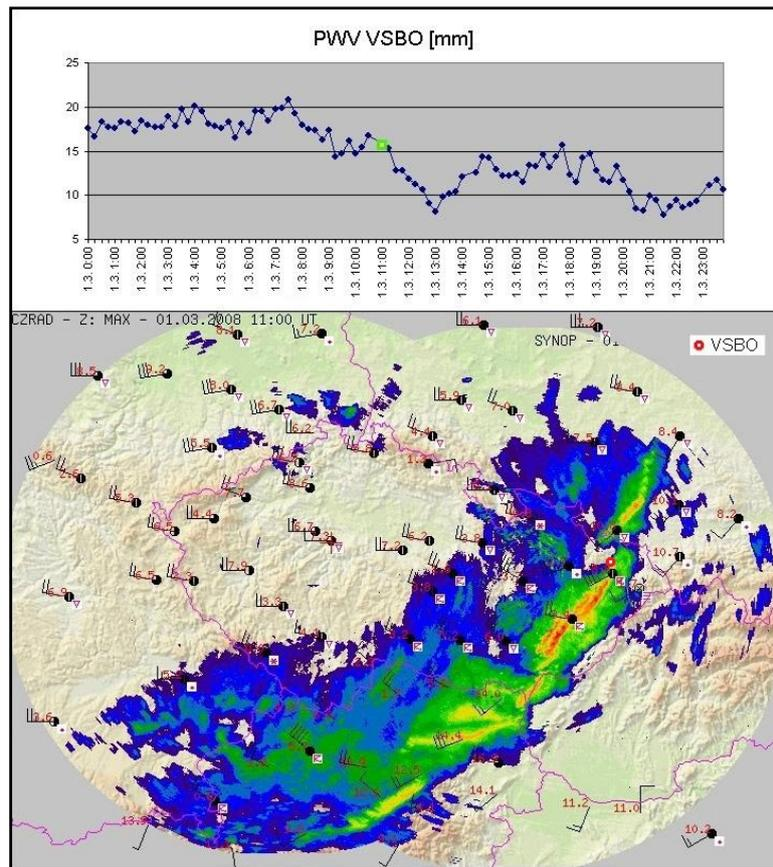
Fig. 5d: Comparison of the results got from GPS measurements at the VSBO reference station with the image from meteorological radar at March 1<sup>st</sup> 2008
