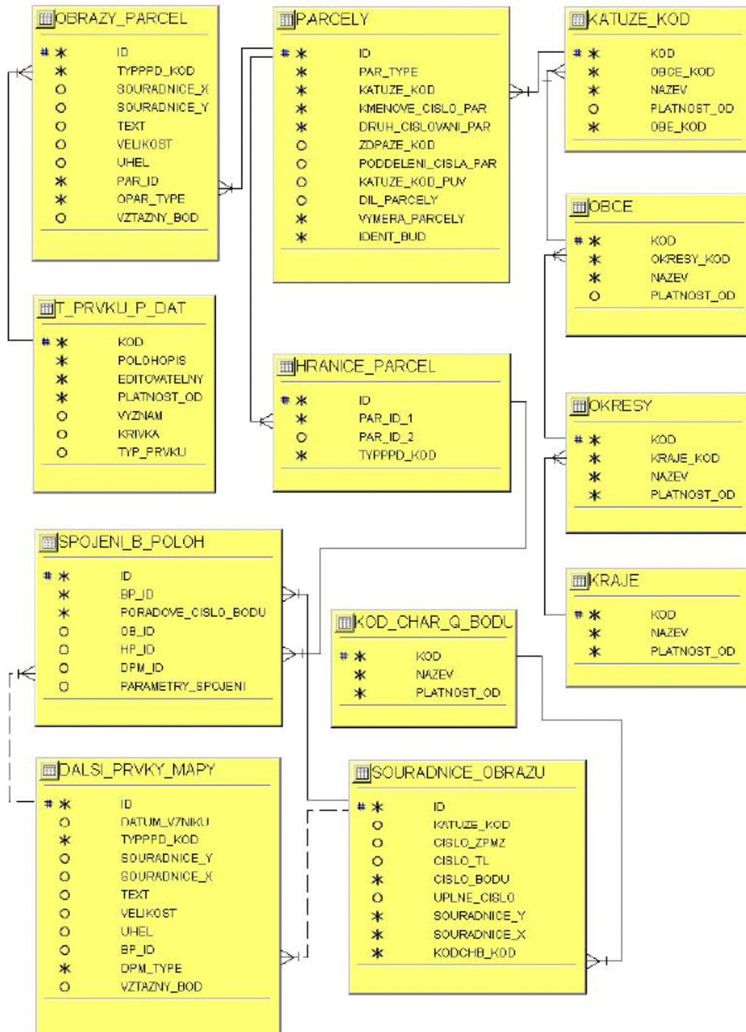
Fig. 1. The part of the data model of the Cadastral Information System for parcels
