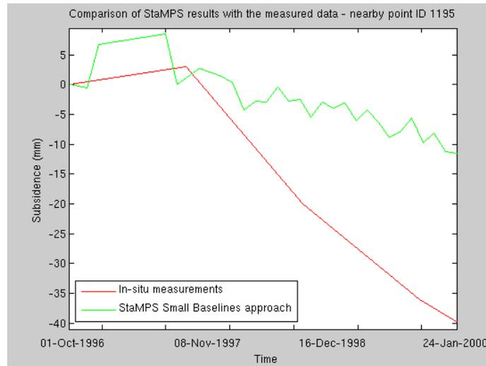
Fig. 3 – comparison of an SB point with a levelling point situated nearby (about 30 m further)
