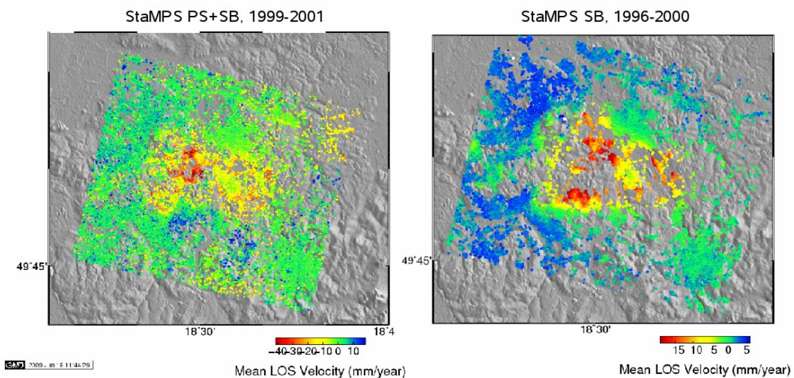
Fig. 2 – PS and SB processing of ERS-2 data using software StaMPS
