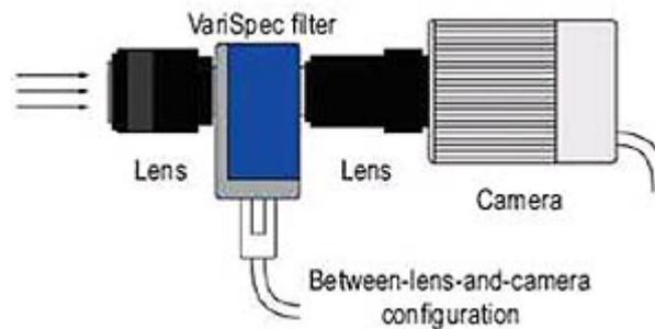
Fig. 4. Configuration of the hyperspectral set: camera, filter and lens
