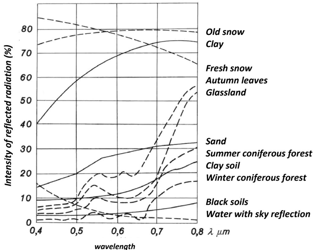
Fig. 1. Spectral response curves of selected natural materials. [6]
