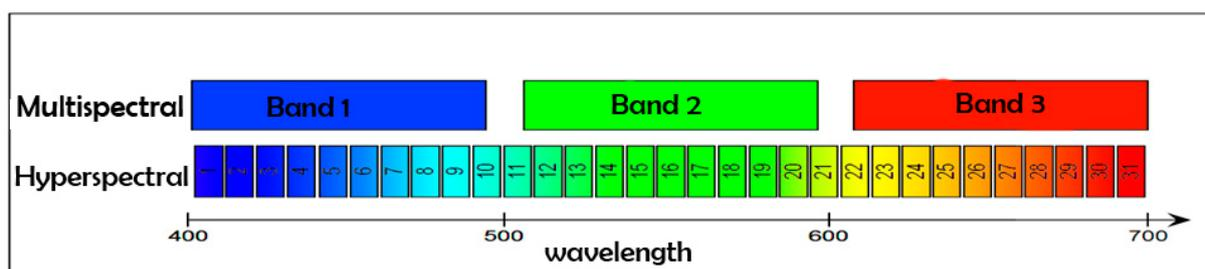
Fig. 3. A comparison of multispectral and hyperspectral bands
