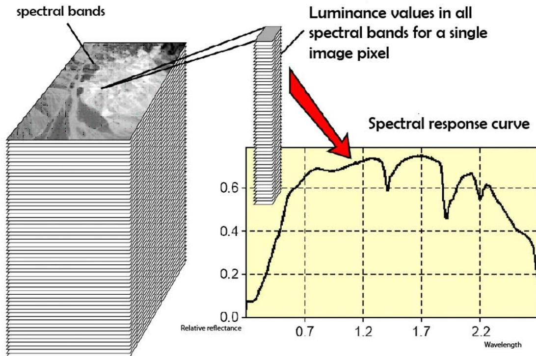
Fig. 2. Acquisition of spectral response curves using a hyperspectral method [5]
