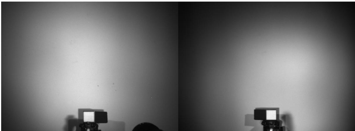
Fig. 7. The effects of vignetting on images acquired using f/4 (left) and f/8 (right) aperture settings.
