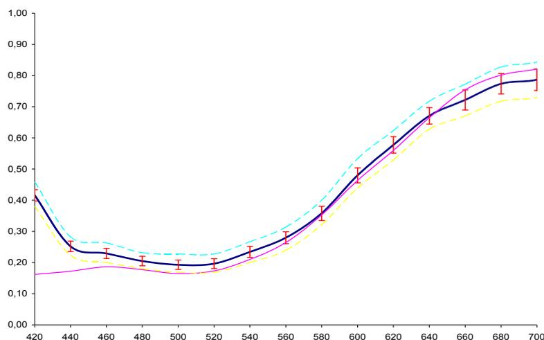
Fig. 6. Characteristic curves for the No 12 sample of the test board – actual values (pink) and hyperspectrally derived values (black). The blue and yellow lines denote the minimum and maximum values of the hyperspectral data.
