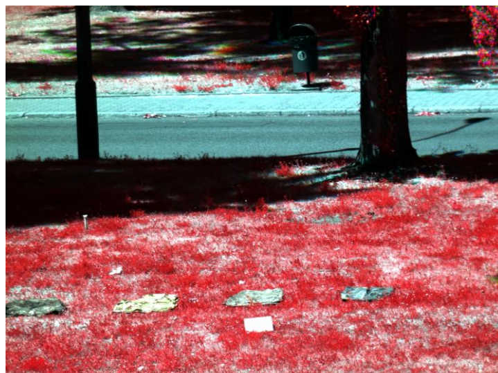
Fig.2. Automatically generated colour composite image composed of the 720nm, 680nm and 660nm bands
