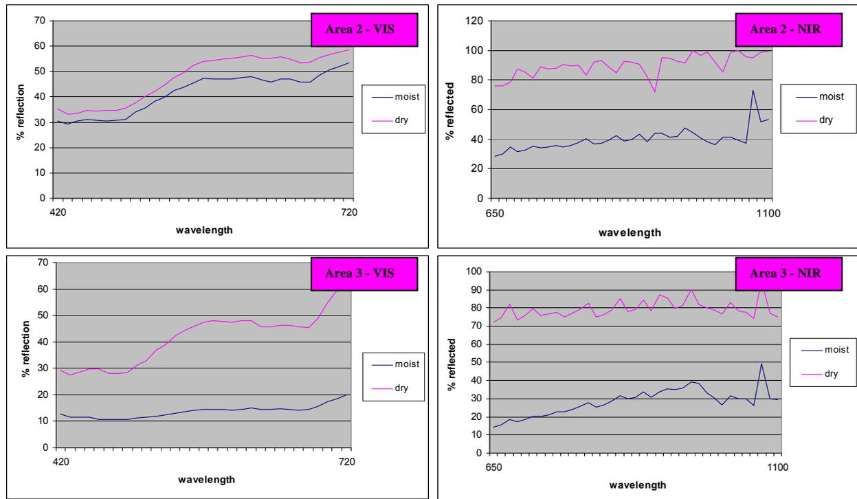
Fig.2. Spectral response curves for 3 areas on the acquired hyperspectral images.
