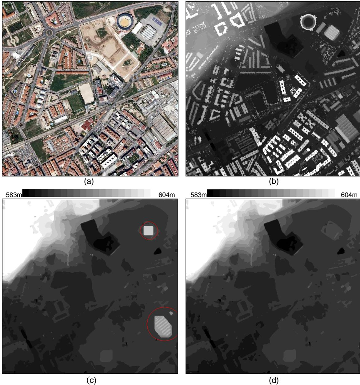
**Fig. 4.** (a) Aerial image, (b) DSM, (c) DTM extracted with the algorithm, (d) MDT extracted with the algorithm and manually cleaned
