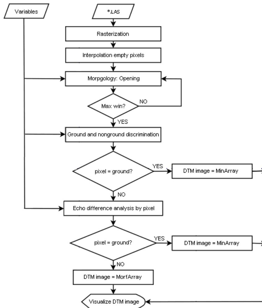
Fig. 1. DTM extraction algorithm from LIDAR data
