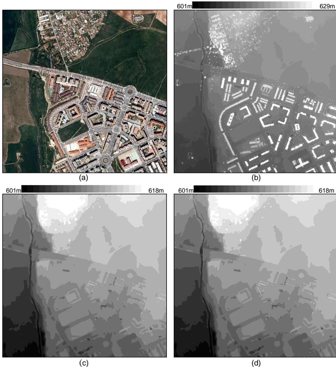
**Fig. 3.** (a) Aerial image, (b) DSM, (c) DTM extracted with the algorithm, (d) DTM extracted with the algorithm and manually cleaned
