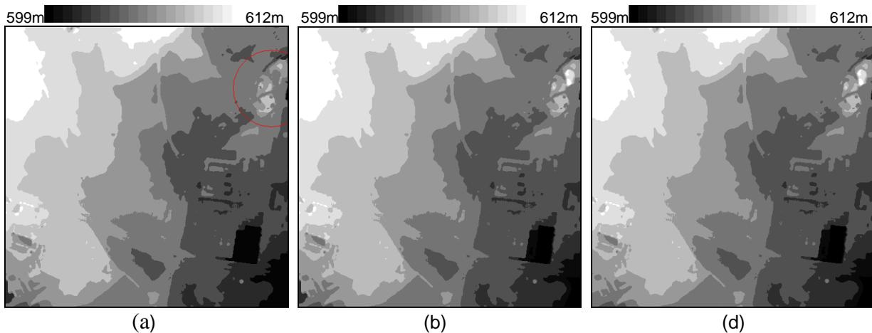
**Fig. 6.** (a) DTM automatically extracted without echo difference analysis, (b) DTM extracted by the algorithm with echo difference analysis, (c) DTM manually corrected
