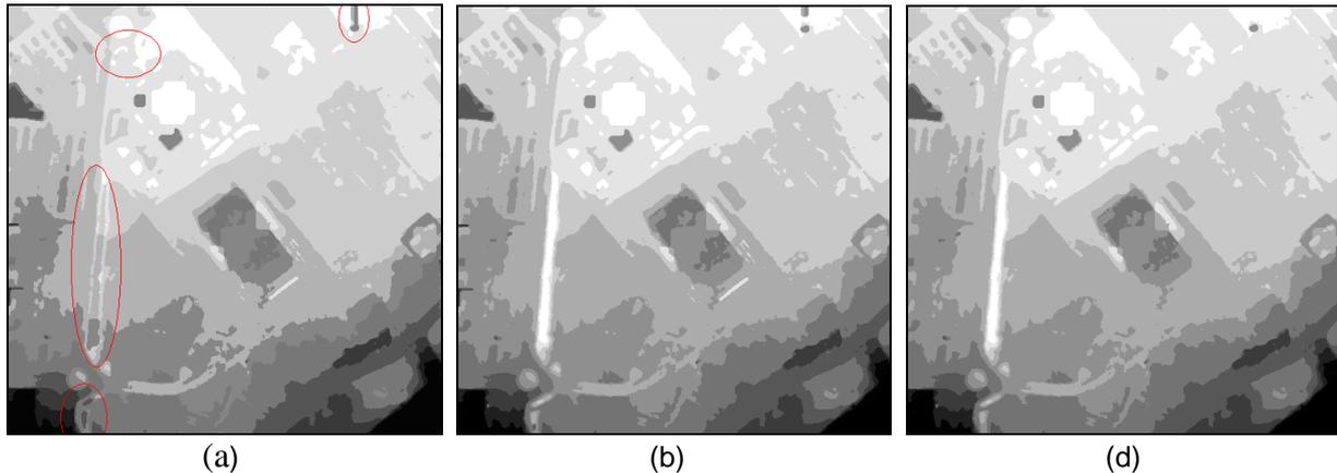
**Fig. 5.** (a) DTM automatically extracted without echo difference analysis, (b) DTM extracted by the algorithm with echo difference analysis, (c) DTM manually corrected
