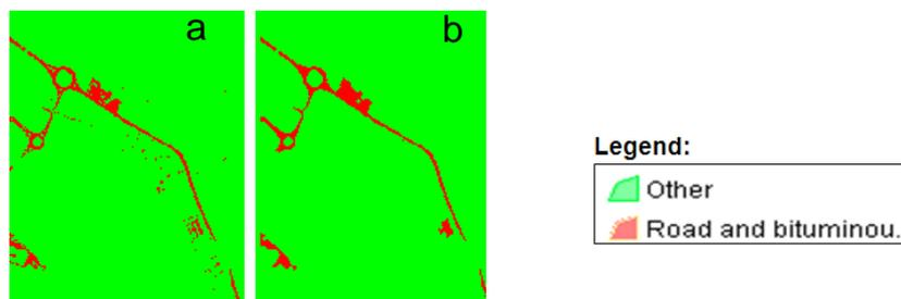
Fig. 6. Pixel-based Classification (step a) and Three-stage Filtering (step b)
