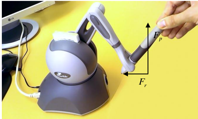
Fig. 2. Low end haptic device (Phantom Omni) used for the test.
