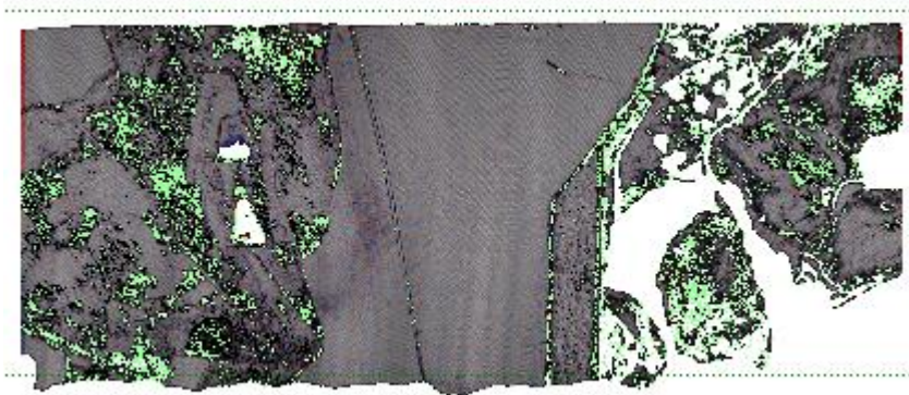
Fig. 5. Difference model (non-smoothed) after strip adjustment
