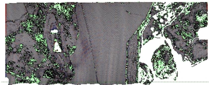
**Fig. 5.** Difference model (non-smoothed) after strip adjustment
