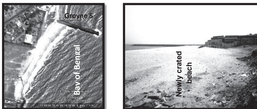
Fig. 4. Field evidence showing accretion south of Groyne – 5.
