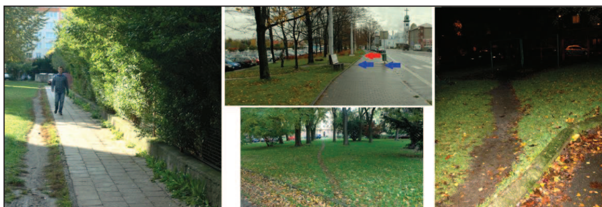
Fig. 3. Left: Maximal pedestrian flow overreaches the capacity of the cobblestone pavement. It caused shortcut in residential district Nové Sady. Middle up: Wrong placement of zebra crossing led to two shortcuts and unused cobblestone pavement in Moravská Ostrava. Middle down: Missing sidewalk around the park force pedestrian walk through the street or shortcut in Poruba part of Ostrava. Right: Playground is not connected with the pedestrian network, thus four shortcuts have been tracked out. (Source: Ivan Mudroň)
