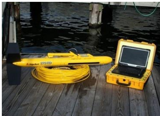
Fig. 3. Side scan sonar system Edgetech 4100
