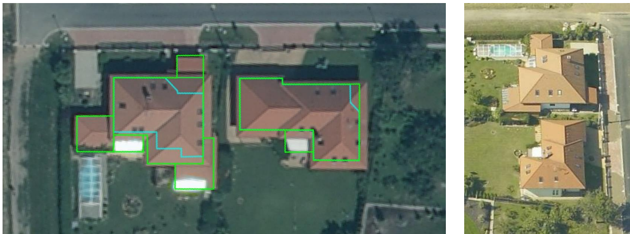
Fig. 1. Left: Orthoimage of two buildings with roof overhangs (green line) over the outer walls (cyan line) Right: Oblique image of the same buildings taken from the east
