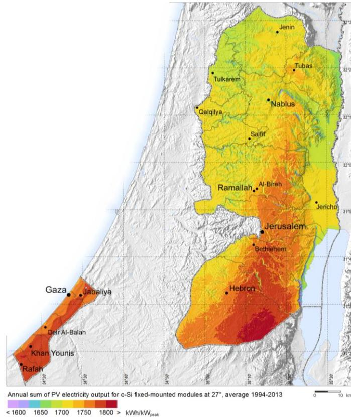
**Fig. 10** Annual PV electricity output from an open-space fixed PV system with a nominal peak power of 1 kW [kWh/kWp].
