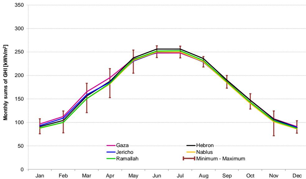
**Fig. 6** Global Horizontal Irradiation - long-term monthly averages, minima and maxima at selected sites. Source: SolarGIS
