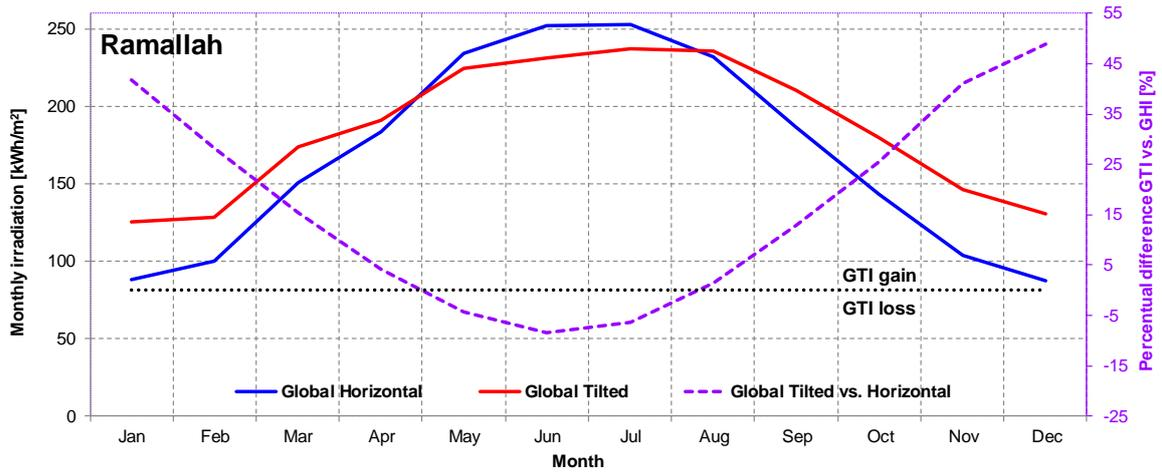
**Fig. 8** Monthly GHI, GTI and Relative gain of monthly Global Tilted Irradiation relative to Global Horizontal Irradiation in Ramallah.
