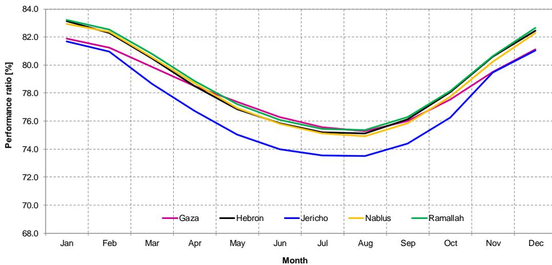
**Fig. 11** Monthly power production from the fixed tilted PV systems at five sites with a nominal peak power of 1 kW [kWh/kWp].
