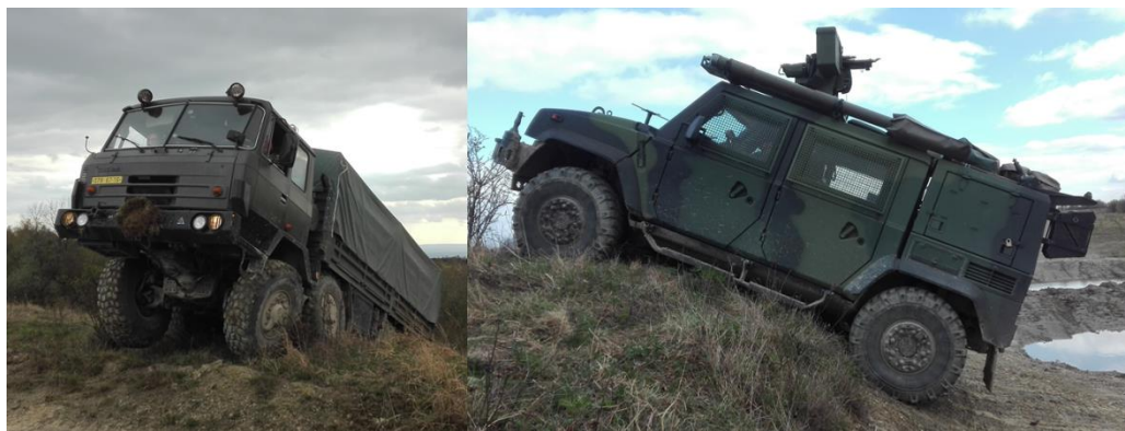
Fig. 3. Vehicles in overcoming microrelief objects during field test
