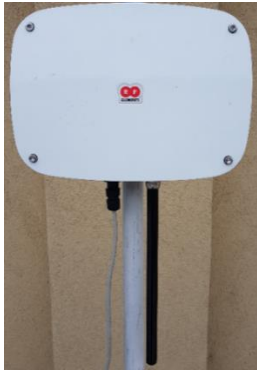
Fig. 5. LoRaWAN gateway built on iC880A concentrator with Raspberry Pi 3.
