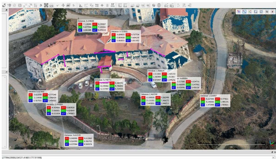
Fig. 5. Measurement of distances of the DJI Phantom 4 Pro Point Cloud (2 nd UAV)
