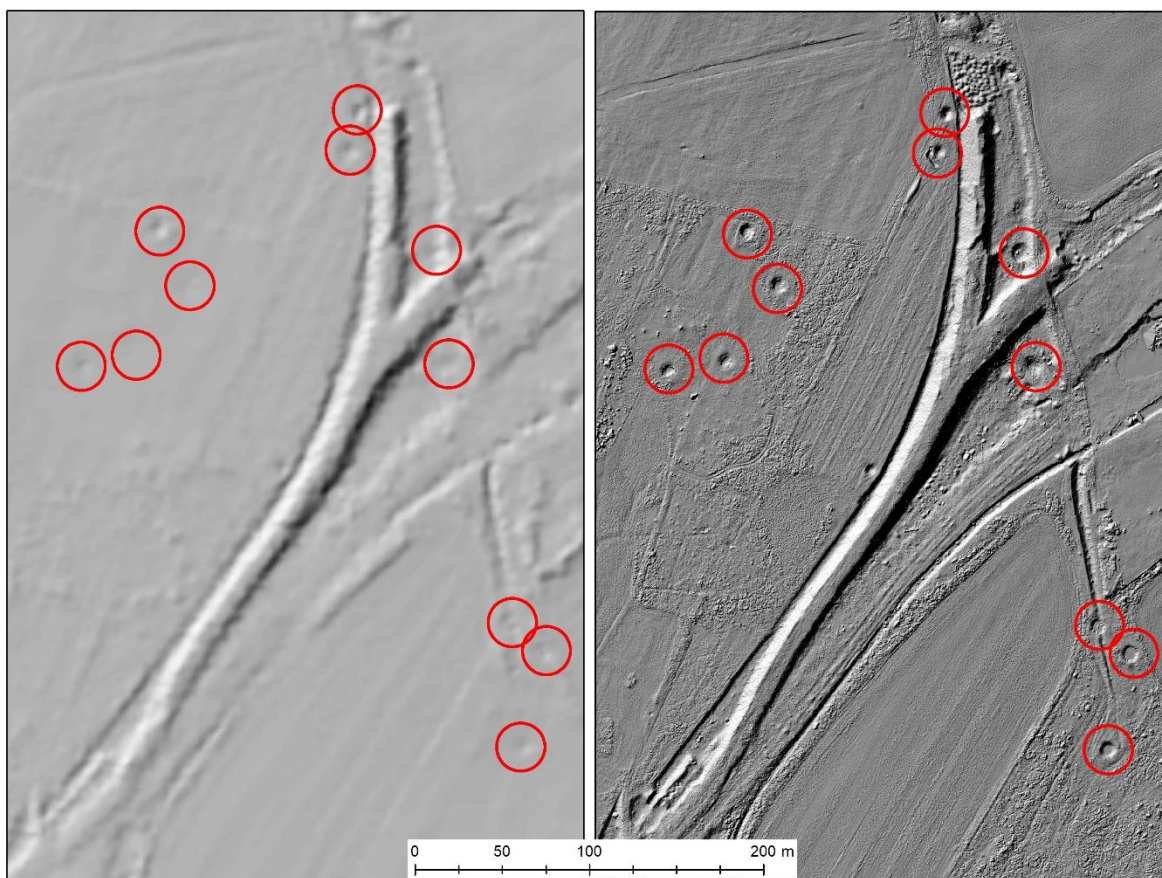
Fig. 3 Craters identified on our LIDAR survey (right) and the same areas identified on the „Digital Terrain Model of the Czech Republic of the 5th generation” LIDAR data available for the whole Czechia.
