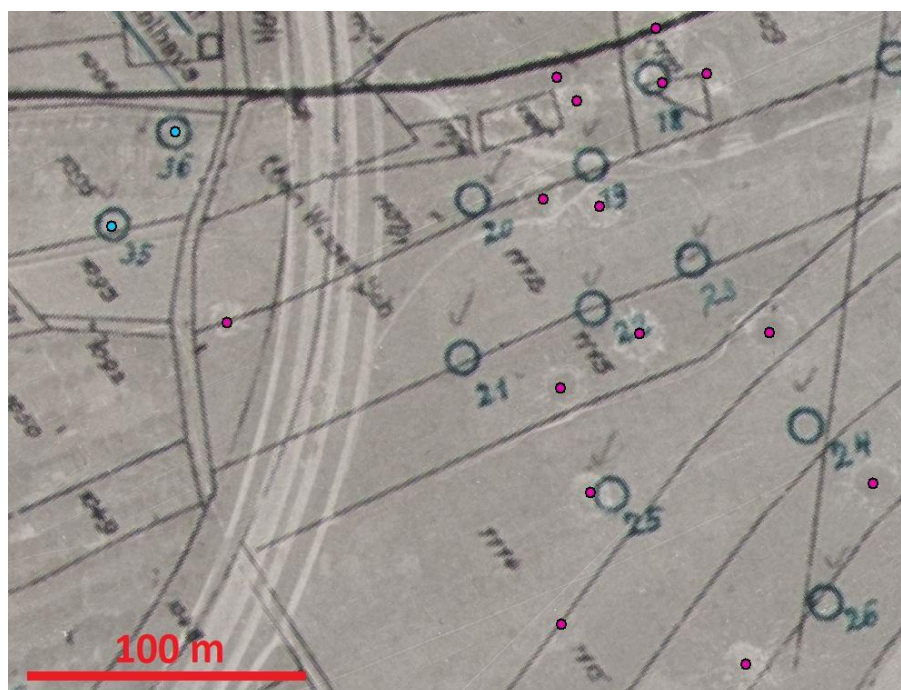
Fig. 2 Crater positions as visually identified after the bombing event into a cadastral map and craters (center points) as identified on corresponding processed archival aerial images
