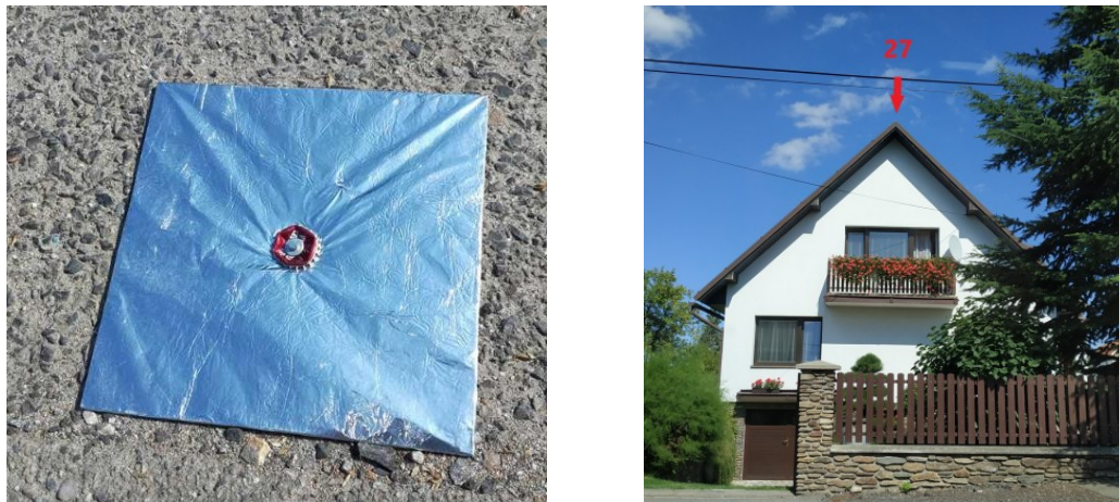
Fig. 2. two types GCP for laser scanning from UAV
