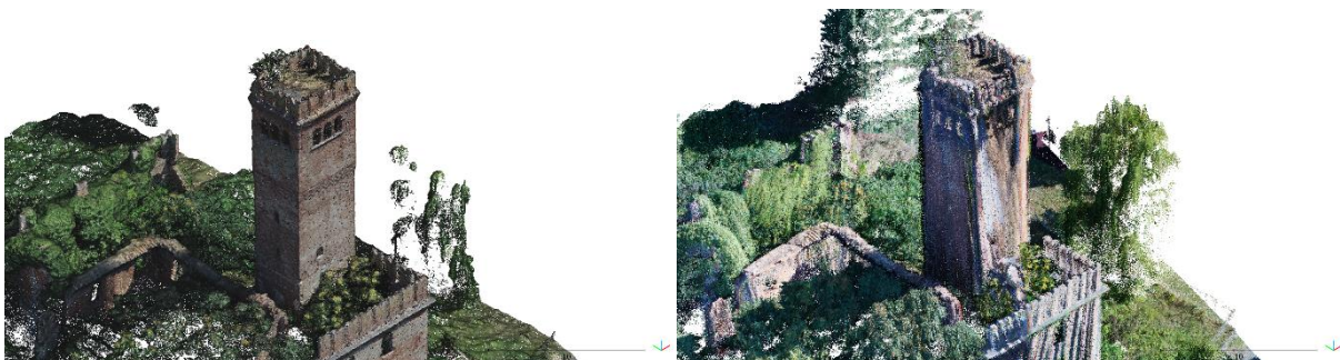
Fig. 5. Overview of the two analysed point clouds: on the left the photogrammetric one, while on the right the one from LiDAR.
