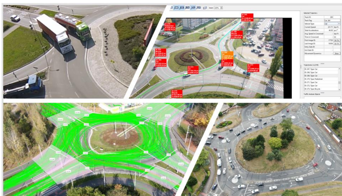
Fig. 5. Conflict situation of lorries, analysis of image of turbo roundabouts and traffic-engineering research on atypical roundabout in England.
